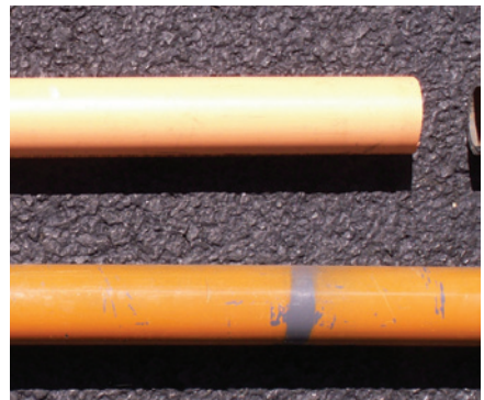
Mix of CPVC and Painted PVC
